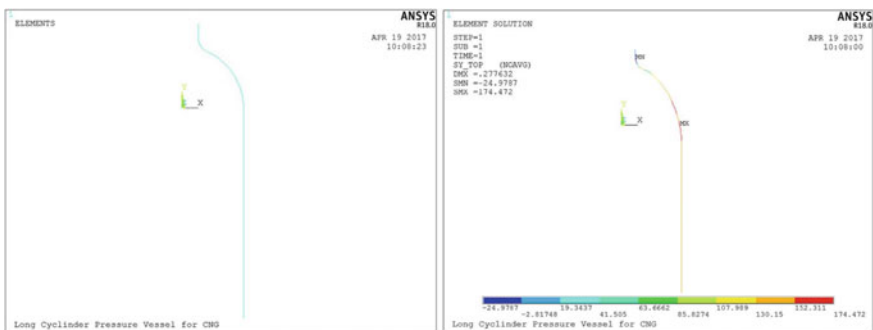
Fig. 7.24 One-dimensional (1D) LF model of the cylindrical pressure vessel
